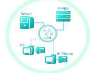
A company office using an IP-PBX
